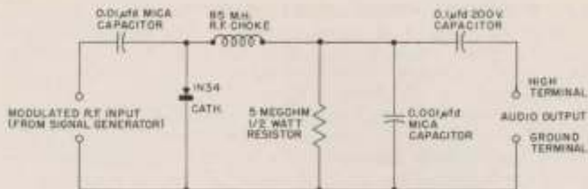
Figure 3-13. AUDIO EXTRACTOR FOR RF SIGNAL GENERATORS
