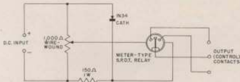
Figure 3-6. TWO-WAY RELAY OPERATING AT TWO DIFFERENT VALUES OF AN INCREASING OR DECREASING DC VOLTAGE
