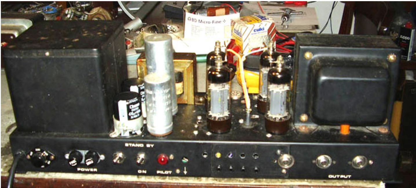
Power amp section showing the new PL36 output tubes in place.
