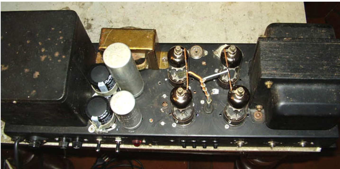
Power amp section showing the new PL36 output tubes in place.
