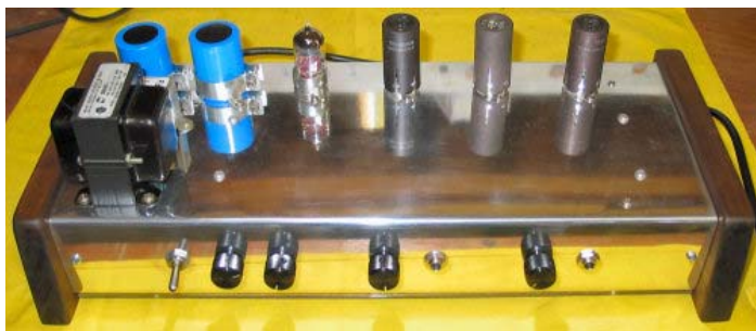
Warbler, a pitch shifting vibrato unit
