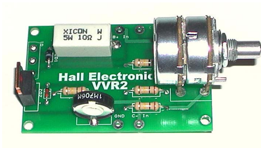
Completed Fixed Bias Board
