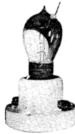
Light bulb with added Electrode
