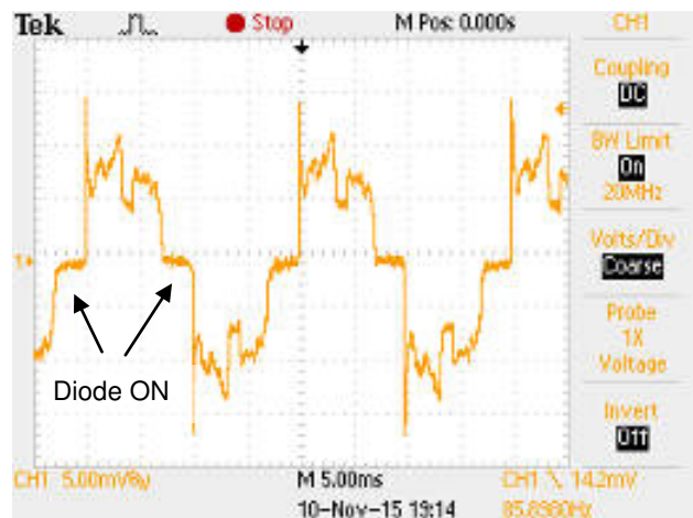
Figure 29. Capacitive coupled signal from wiring
